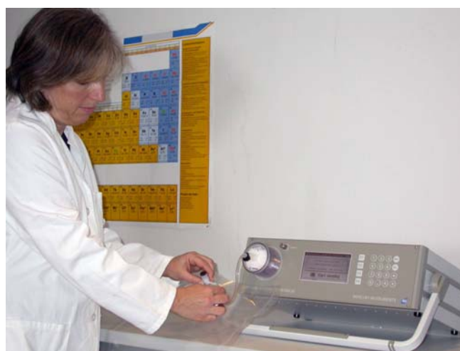
Opening of the valve to release sample into the analyzer
