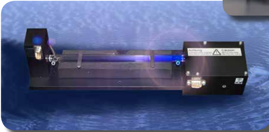
The soul of the machine: The optical bench inside the VM-3000
