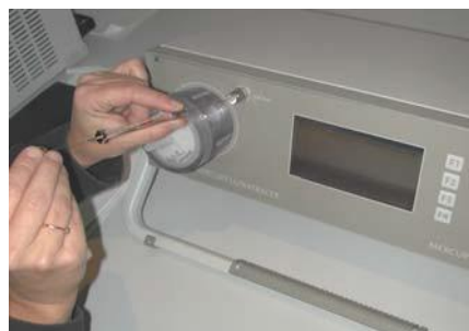
Injection of calibration gas into the calibration port of the analyzer
