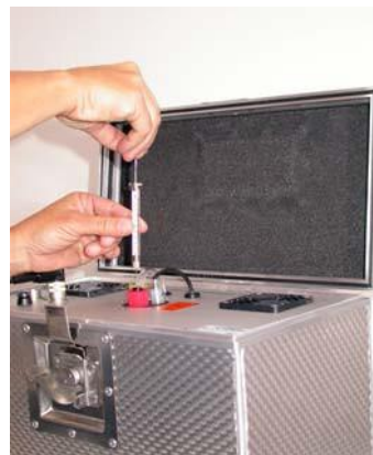
Extracting calibration gas from the UT-3000 calibration device
